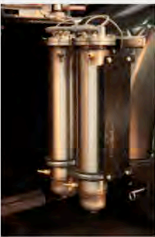
Hydrogen Injection Technologies’ aftermarket supplemental hydrogen on-demand fuel system.
