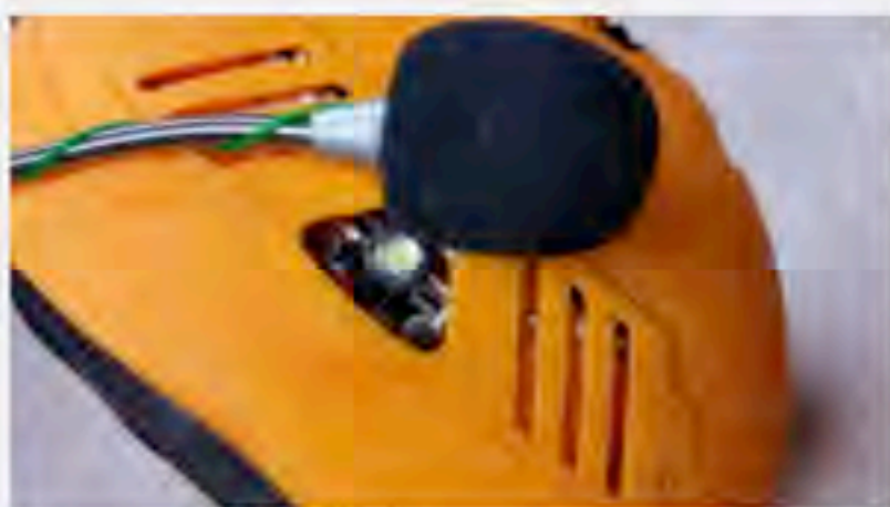
A built-in LED light on the Smart Helmet controllable through the smartphone app.
