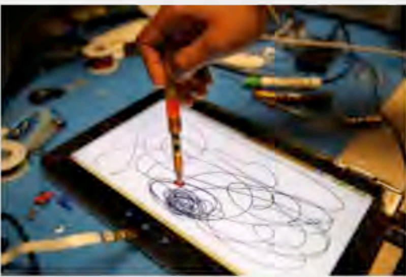
An NFC stylus that’s able to charge wirelessly from the tablet
