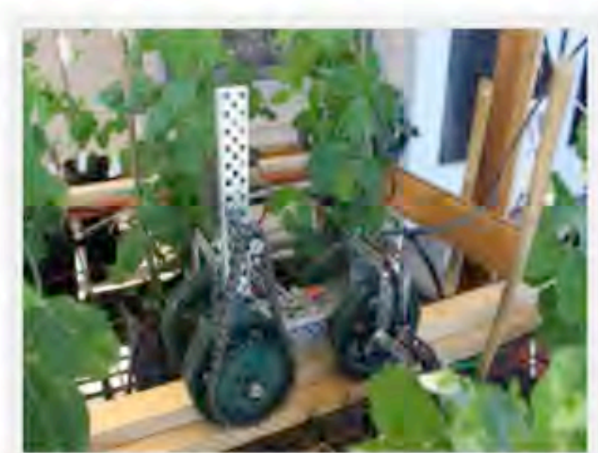
A robot, controlled by a BeagleBone Black development board, was outfitted with water and solenoid valves to deliver precise amounts of irrigation to the peas.
