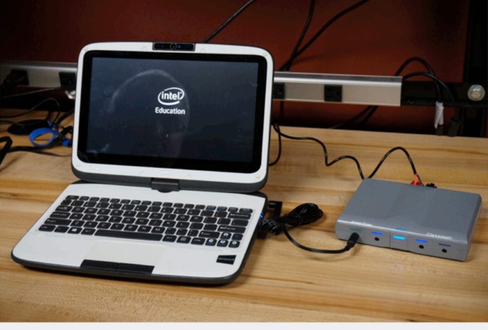
A Classmate PC charging from a near-final version of the SSC, each of which can charge up to four laptops at once when supplied with adequate power from the solar panel.
