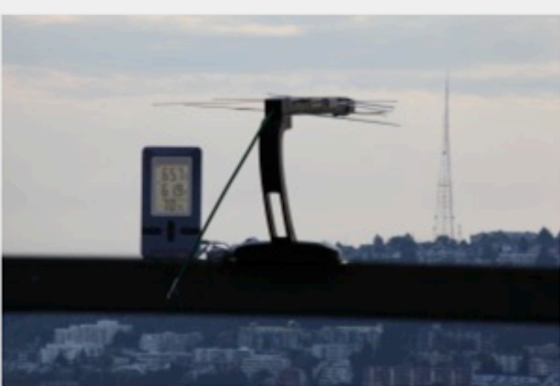
A kitchen thermometer, with LCD display being powered by RF signals from a TV tower 4 km away. Photo: University of Washington
