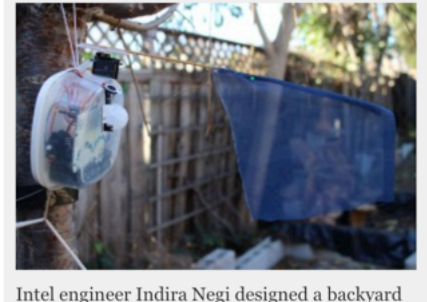
Intel engineer Indira Negi designed a backyard “squirrel chaser” that uses an Arduino, infrared sensor and servo motor.
