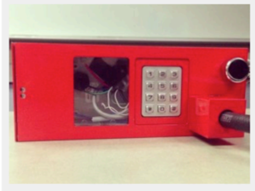
Prototype of IoT bike sharing device which is attached to a bicycle – part of OBI version 2.0 bike sharing development.
