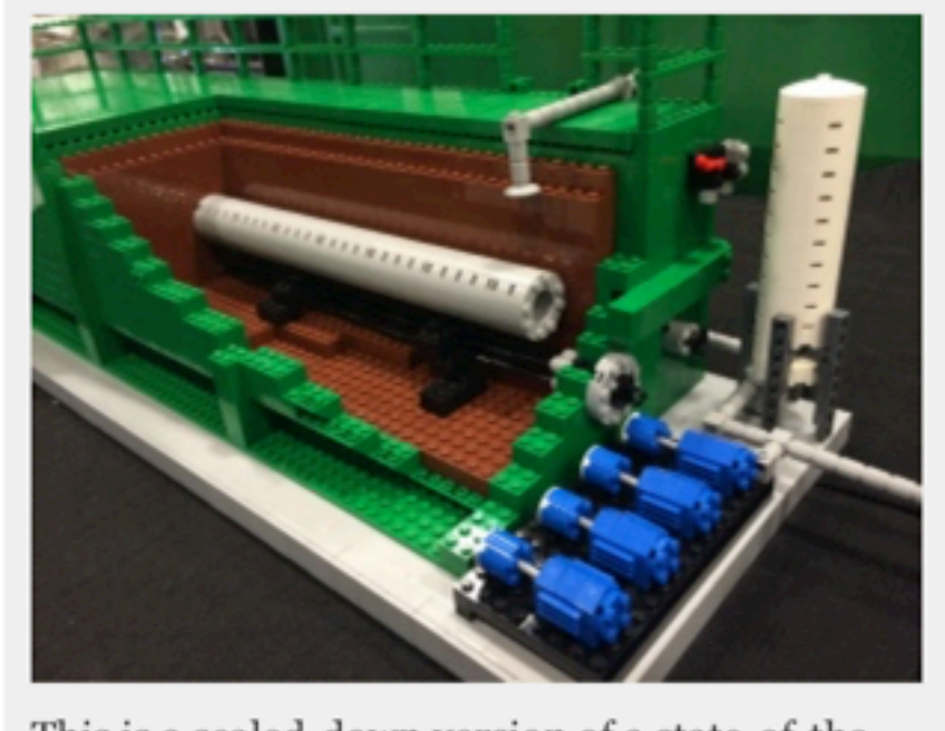
This is a scaled-down version of a state-of-the-art pipeline simulator known as the External Leak Detection Experimental Research (ELDER) test apparatus. It is being used by TransCanada to test the different Cable Based Leak Detection technologies in a unique Joint Industry Partnership with fellow pipeline operator Enbridge and the Governments of Alberta and Canada. Photo credit: TransCanada Corp.
