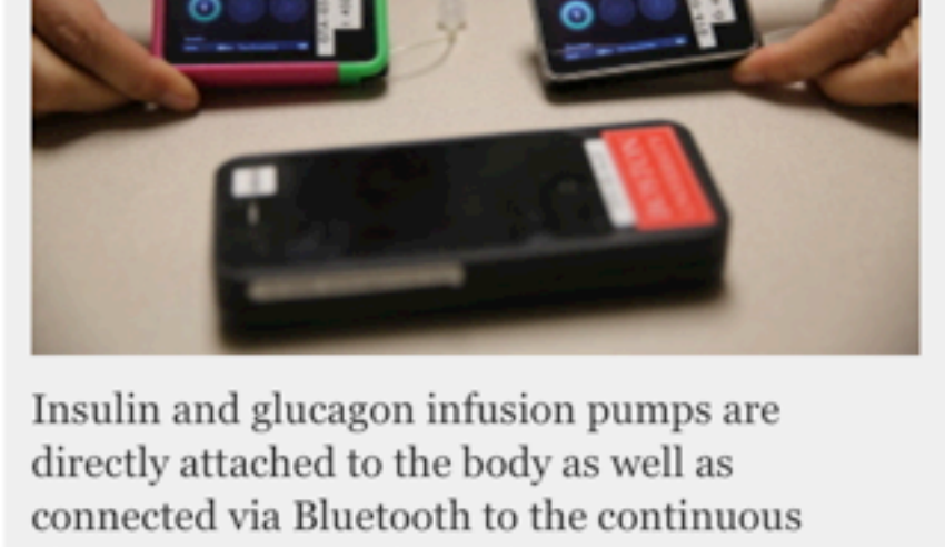
Insulin and glucagon infusion pumps are directly attached to the body as well as connected via Bluetooth to the continuous glucose monitor and an iPhone.
