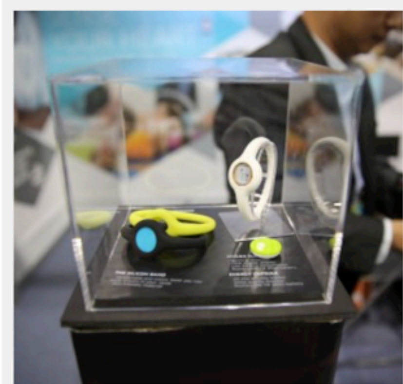
The $79 Maxwell Guider Technology Power Watch is powered by disposable coin batteries and uses an e-Ink display.
