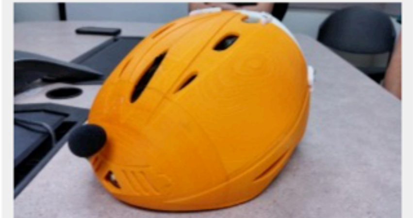
3D printers helped to create the outer shell of this smart helmet prototype.
