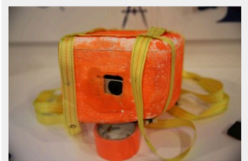
The styrofoam casing insulated and protected the technology from extreme temperatures and a crash landing on its trip to and from near space.
