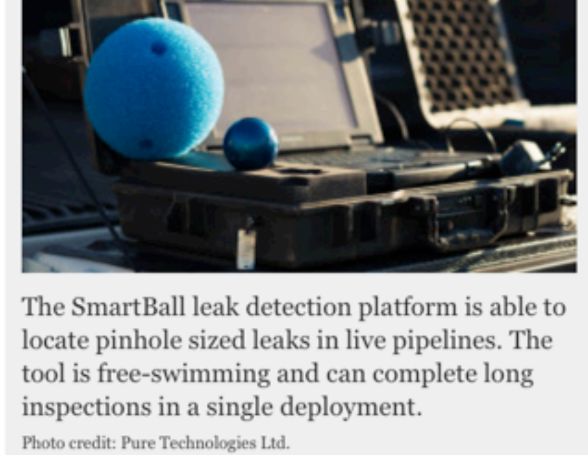
The SmartBall leak detection platform is able to locate pinhole sized leaks in live pipelines. The tool is free-swimming and can complete long inspections in a single deployment. Photo credit: Pure Technologies Ltd.
